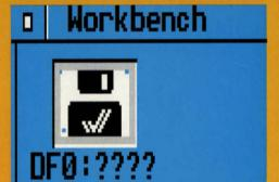
If the disk hasn't been formatted (if it's brand new or is in another computer type), the Amiga will call it 'DF0:????'. Click once on the disk icon, press the left mouse button and select (click the left mouse button on) the Format Disk option from the Workbench icons pull down menu
