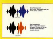
this is best done by ear, listening for when the loop sounds right. However, for sustained sounds, you have to make sure that the sound level at the start of the loop is as close as possible to the level at the end of the loop, otherwise you will hear a nasty click every time the loop is played.
