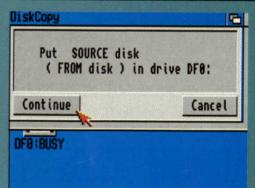
Wait for a couple of seconds until the Amiga starts reading the contents of the disk that you want to copy into its memory. The disk will be copied on a fast track-by-track basis.
