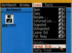
Once the 'INSERT DISK TO BE FORMATTED request box appears on the screen, remove the Workbench disk from the disk drive and insert the disk that you wish to format.
