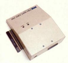
The Trumpcard hard drive: you can plug it on the edge of an A500 or stick it inside an A2000.
