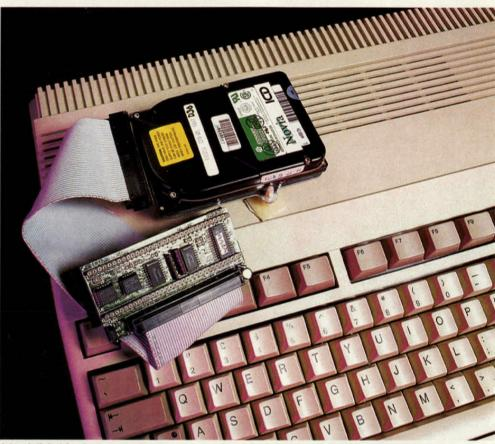
A hard disk drive has many advantages over a floppy disk, but the main ones are that you can save programs straight to the hard drive, so you don't have to worry about disk swapping, and you've got much more storage space, which is particularly useful with memory-intensive programs such as graphics.
